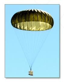
The G-14 cargo parachute provides the capability to deliver non-fragile supplies and equipment using a lowvelocity air delivery method. In its basic configuration, it is capable of supporting and delivering up to 500 lbs; however, when in a cluster of three (3), it can support payloads up to 1,500 lbs. The assembly includes a canopy, static line, pack and drogue. The overall assembly weighs approximately 37 lbs.
